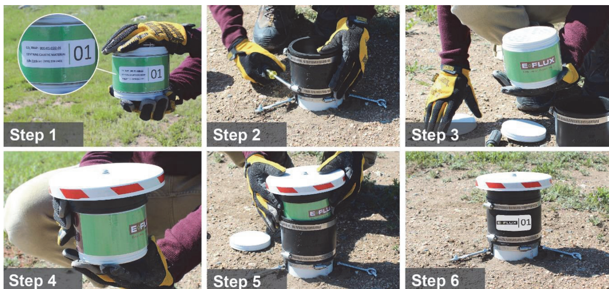
Figure 3. In-ground Receiver Installation (Steps 1,3,4,6-8).
